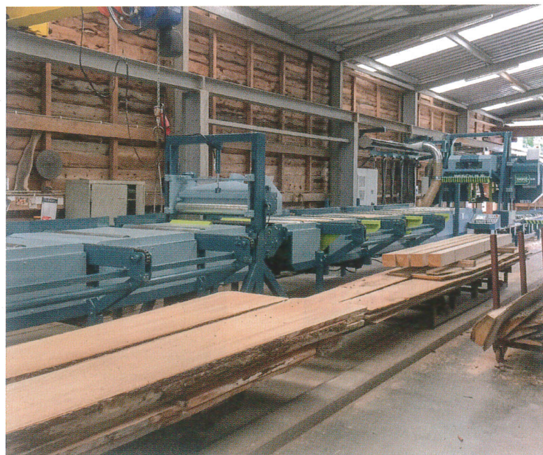
A new ES 1200 Compact stationary band saw has been running in Netherlands with Inlands Hout Van Leersum
